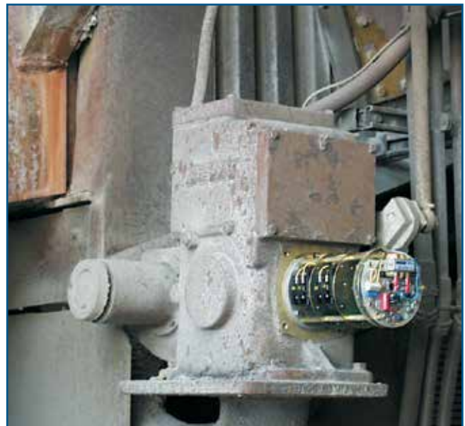
Group 11 actuator with the gasketed control end cover removed.
