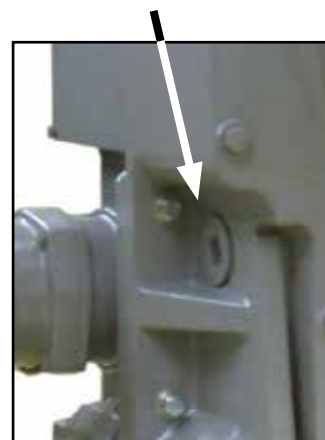
GEAR INSPECTION PLUG
