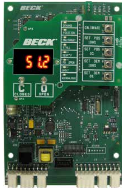
DCM-2 with Feedback Display Part No. 22-5011-44
