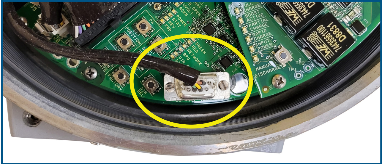
GROUP 57 WI-FI DB9 CONNECTOR (J20) ON THE DCM (shown equipped with optional Backup Power Unit (BPU))
